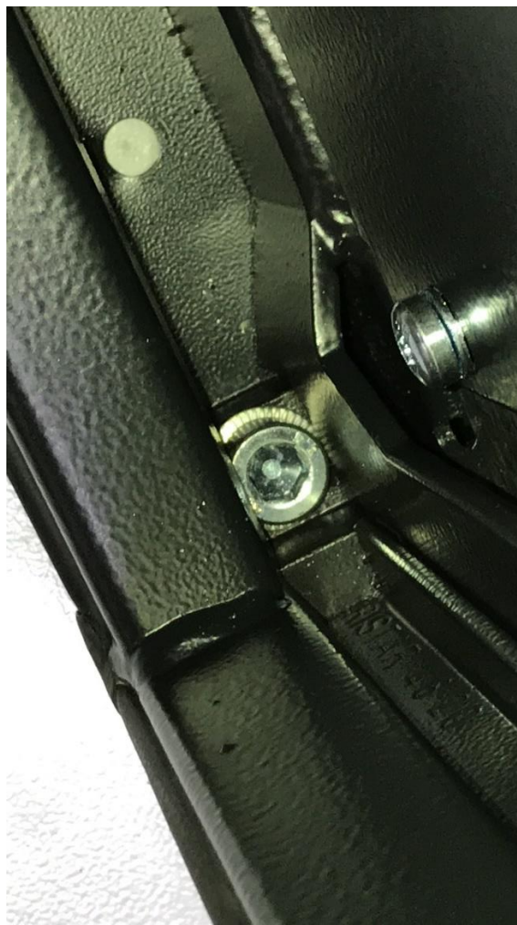
Contact washer M10 / hexagon socket M10 (8.8)
