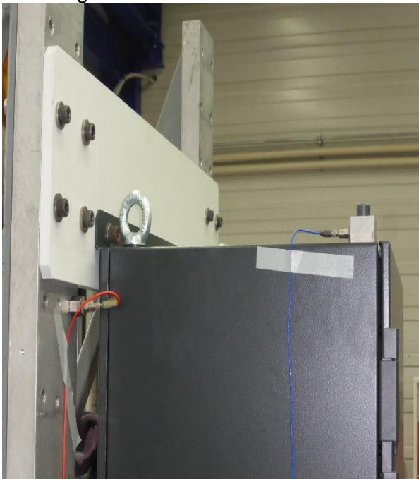
Photo No.11 / measuring sensor (right) and control sensor 1 ( left )
