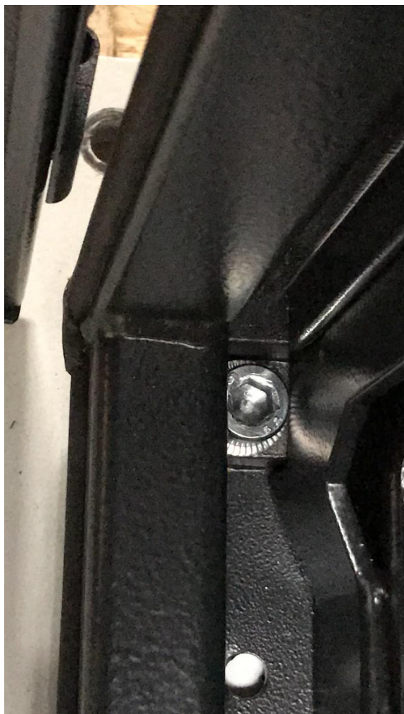
Contact washer M10 / hexagon socket M10 (8.8)
